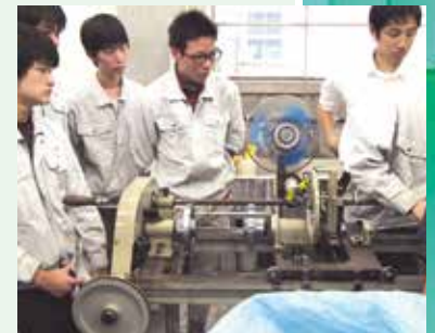
工学実験 (ねじり試験) Mechanical Engineering in Experiments (Torsional Test)
