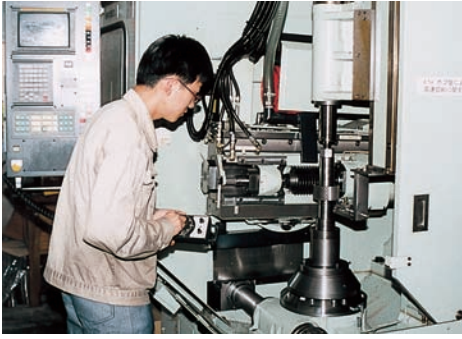
歯車の高速ホブ切り high-speed gear hobbing
