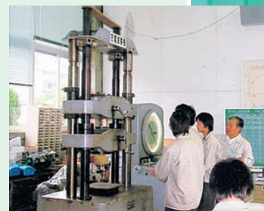
工学実験 (引張実験) Experiments in Mechanical Engineering (Tension Test)
